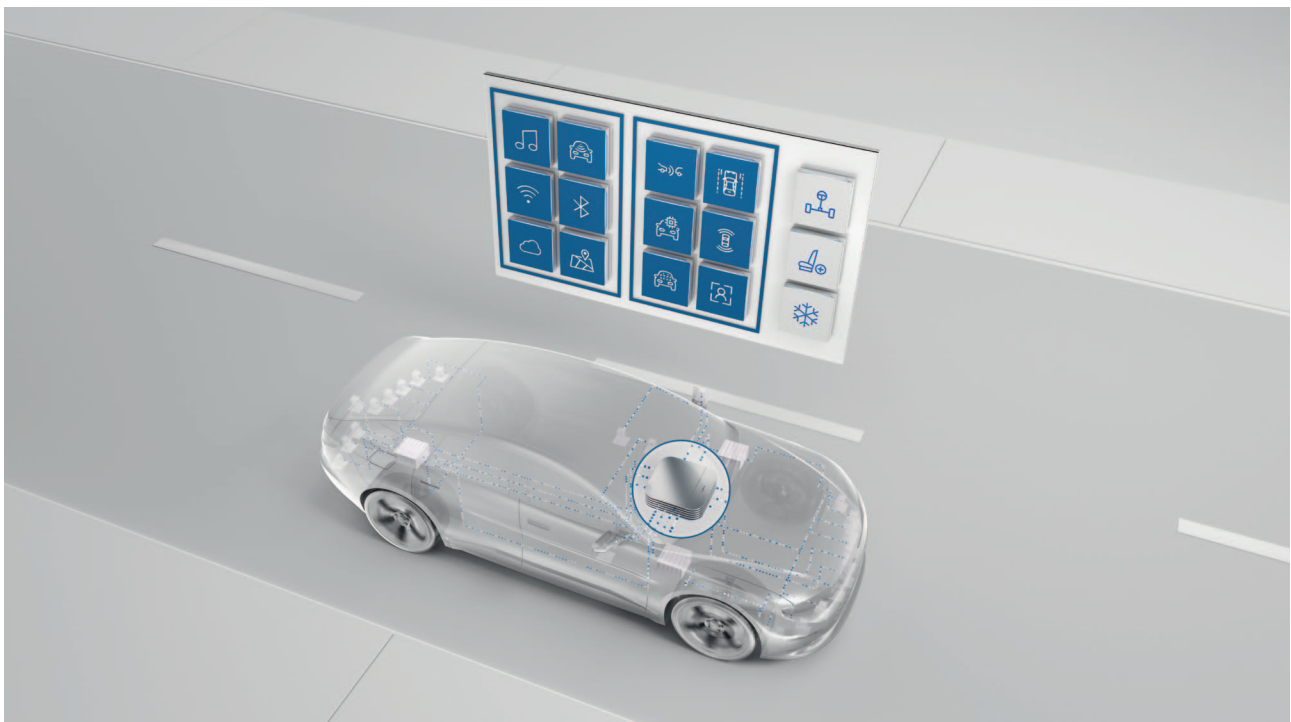
Figure 12: Centralized apps in the vehicle computer with high speed access to the sensors and actuators.
